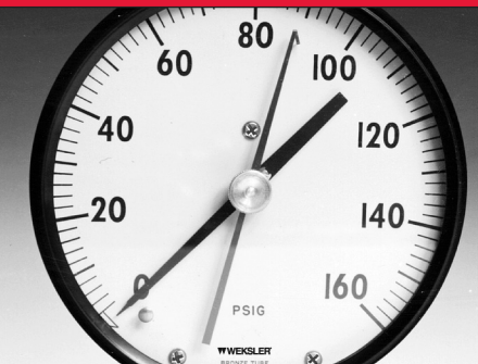
Maximum Pointer available for gauges 4½" size and larger. Indicates maximum pressure attained. Can be reset by a knob on outside of window.
